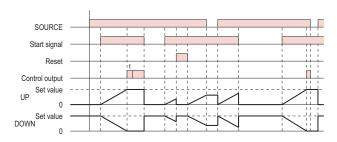
Timing starts when the start signal goes ON, and is reset when the start signal goes OFF.
