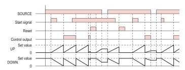
Timing starts when the start signal goes ON.
