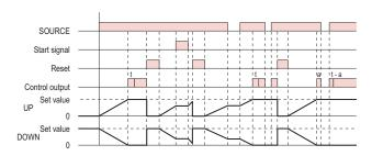
Timing starts when the reset input goes OFF.
