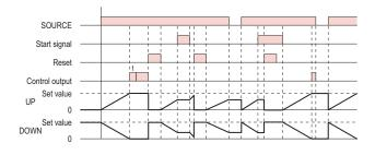
Timing starts when the reset input goes OFF.
