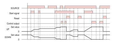
Start signal enables timing (timing is stopped when the start signal is OFF or when the power is OFF)
