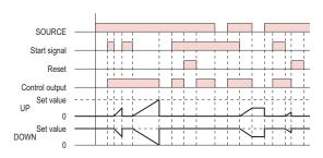
The control output is ON when the start signal is ON(except when the power is OFF or the reset is ON).
